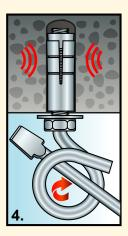
Tighten firmly hook up the washer, with a screwdriver.
