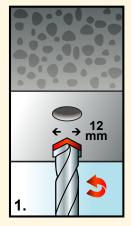
Drill 2 holes to a depth of 7 cm. Diamond drill bit, diameter 12mm.
