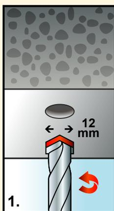
1. Drill 2 holes to a depth of 7 cm. Diamond drill bit, diameter 12mm.
